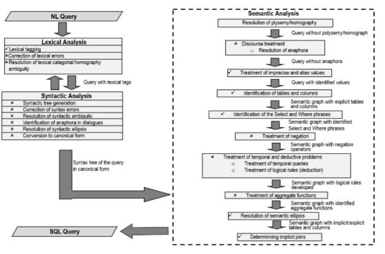
Fig. 2. Functionality layers of the translation module.
